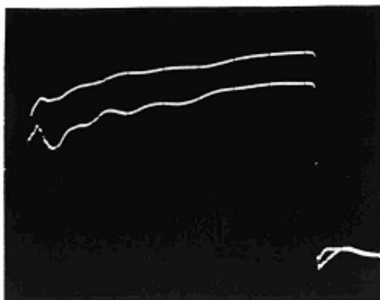
(c) High resistance joint (32n) near one end of winding.
