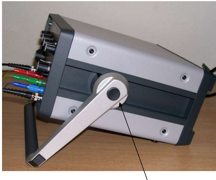
Figure 2.9 Handle pivot buttons (one on each side)
