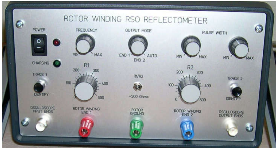
Figure 2.4 Reflectometer front panel controls (TDR100RB)
